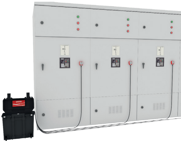
Precedence Detection Locate PD in MV metalclad air-insulated switchgear by determining which sensor PD signals arrive at first.
